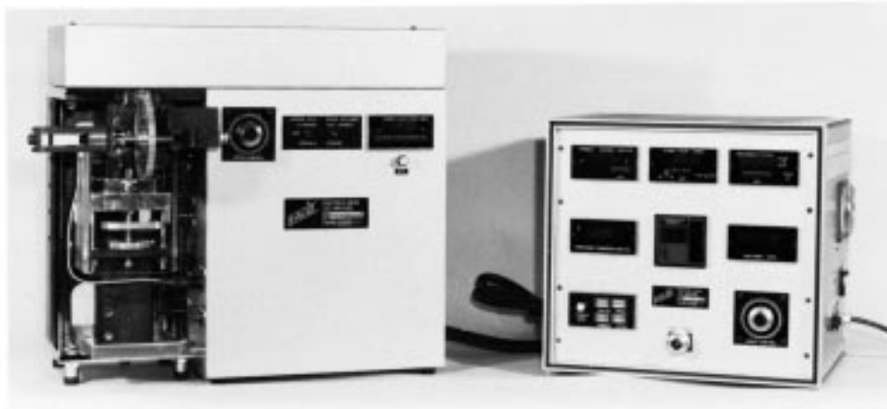
FIG. 2 Falex Digital Pin and Vee Block Test Machine
