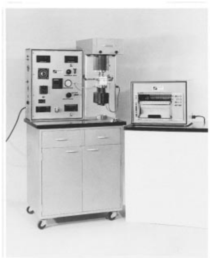
FIG. 3 Falex Variable-Speed Four-Ball Wear Test Machine
